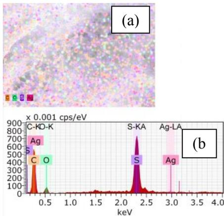
**Fig.2 (a) FESEM of the Ag-PSf membrane, (b) EDS graph of the Ag-PSf**
