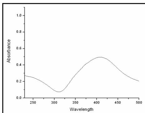
**Fig.3. UV-Vis absorption spectrum of Ag nanoparticles**
