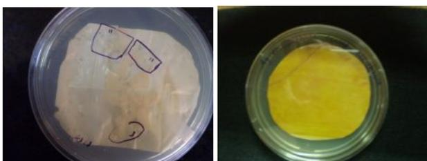
**Fig.6 (a) Biofilm on PSf (b) Absence of biofilm on Ag-PSf**
