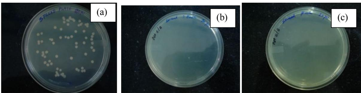
**Fig.5 (a) Culture plate inoculated with unfiltered water (b) Culture plate inoculated with water filtered with PSf membrane (c) Culture plate inoculated with water filtered with Ag-PSf membrane**
