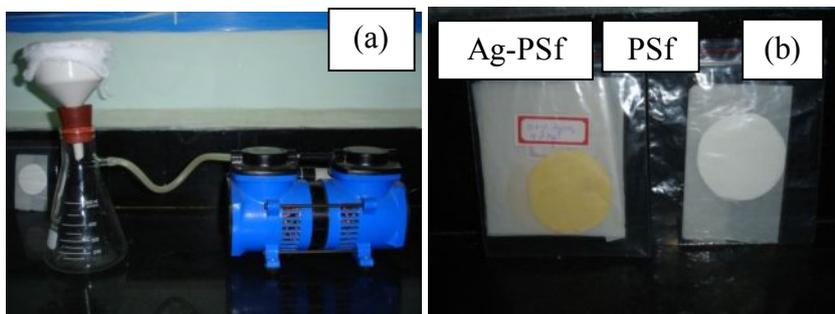
**Fig.4 (a) Filtration unit, (b) PSf and Ag-PSf membranes**
